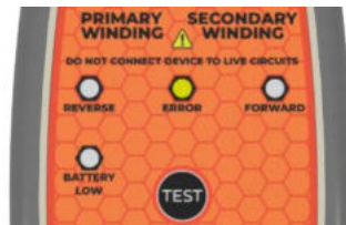
Figure 1.5 Amber LED 1 second flash
