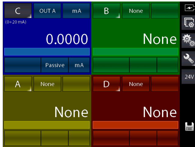
Figure 45 – Setting the mA-loop generation
