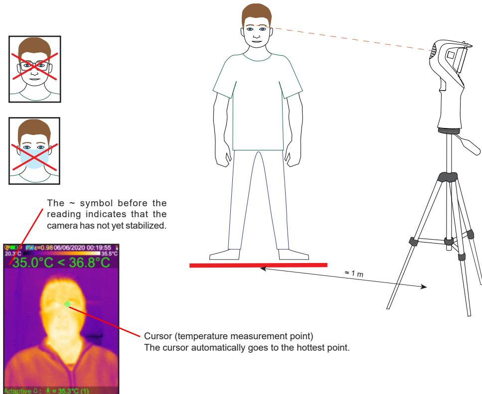
If the alarm is triggered, check that the cursor is in fact on the corner of the person's eye or on their forehead. If it is placed on the neck, the person must hide their neck with their hand.
