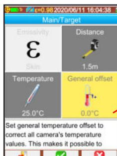
Set the general offset (temperature difference between the forehead and the internal temperature) to 2°C.
