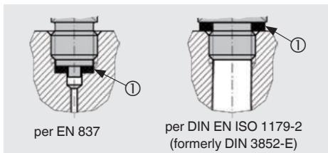
Correct sealing of the process connections with parallel threads at the sealing face ① must be made using suitable flat gaskets, sealing rings or WIKA profile sealings.
