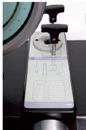
Control schematic on the CPP4000-X instrument base
