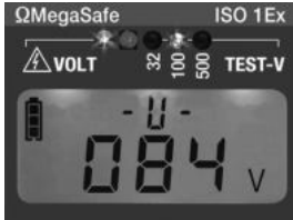
Charge voltage indication with external connected capacitance
